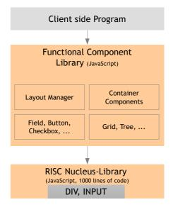
On the bottom layer, the two primitive elements are encapsulated by some "Nucleus Library". This library provides an API that allows some access to the primitive elements.
