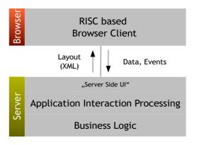
The development and interaction processing of dialogs is located on server side. Result: the server side interaction has direct access to the server side business logic. - The front-end client is a generic rendering engine, receiving form descriptions (XML) from the server side, rendering them and passing events and data updates back to the server side.
